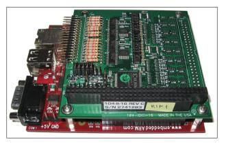
A typical PC104 stack with a single board computer (SBC) and an interface card. The SBC has built in serial ports, Ethernet adapter and USB ports.
