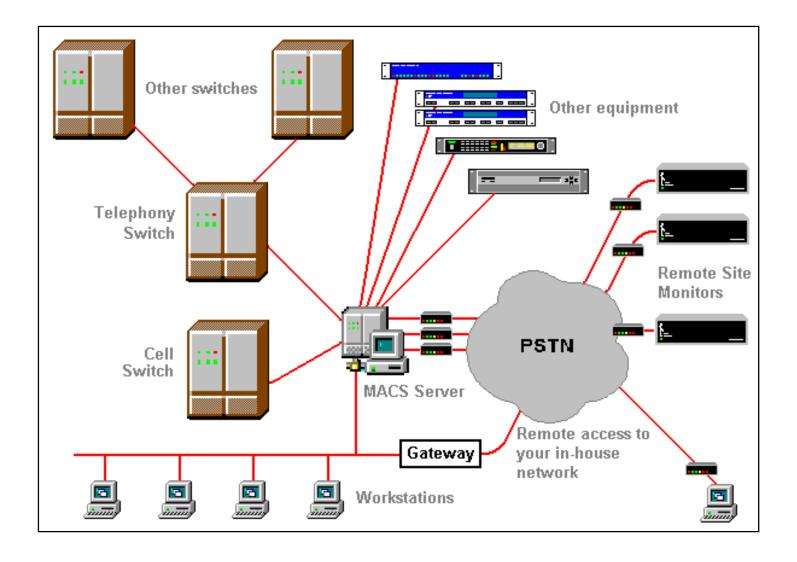
**Micus Alarm And Control System (MACS)** is a computer based system which configures, controls and monitors various pieces of equipment, and collects and processes alarms generated by the equipment.
