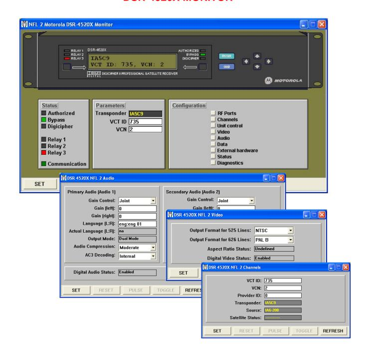
The Motorola DSR-4520X is an advanced featured DigiCipher® II integrated receiver/decoder (IRD). The Motorola DSR-4520X digital satellite receiver is designed for cable and other commercial satellite operators who want to maintain their signal in a digital format.
