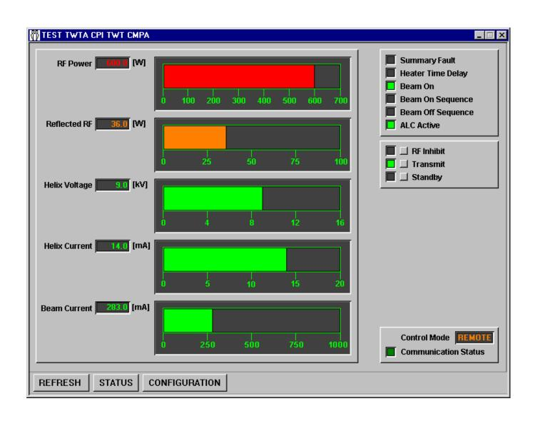
CPI TWT amplifier (TWTA) is used in satellite communications earth stations, satellite news-gathering vehicles and fly-away applications operating in the C and Ku frequency bands. *Micus Alarm and Control System (MACS)* provides automated alarm monitoring and remote control access to any number of TWTAs from one or more computer workstations on your computer network.
